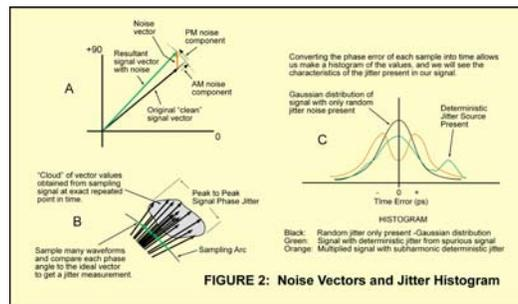
Figure 2: Noise Vectors and Jitter Histograms (Click on image to enlarge)
