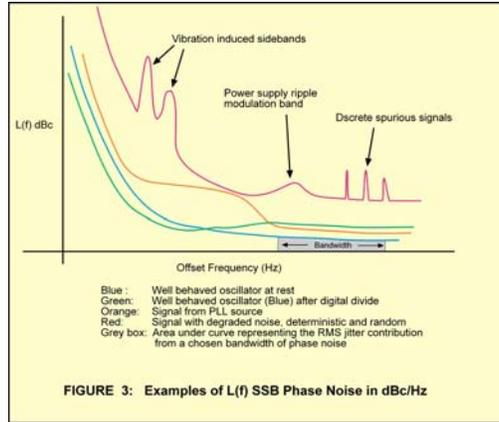
Figure 3: Examples of L(f) SSB Phase Noise in dBc/Hz (Click on image to enlarge)
