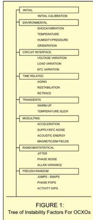
Figure 1: Tree of Instability Factors for OCXOs (Click on image to enlarge)
